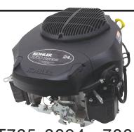
• New, Kohler KT735-3094 7000 series four-cycle, twin-cylinder, air-cooled, vertical shaft, gasoline, OHV, with cast iron cylinder sleeves. Applications include residential riding and zero turn mowers. Fits TimeCutter, TimeCutter Max and Quest S. Does not include fuel tank or muffler. Adjustable mechanical governor.
